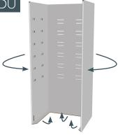
Fold unit out from flat. Fold the base flaps under
