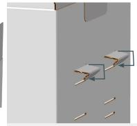
Tab through the top slots, before returning through the bottom slots.
